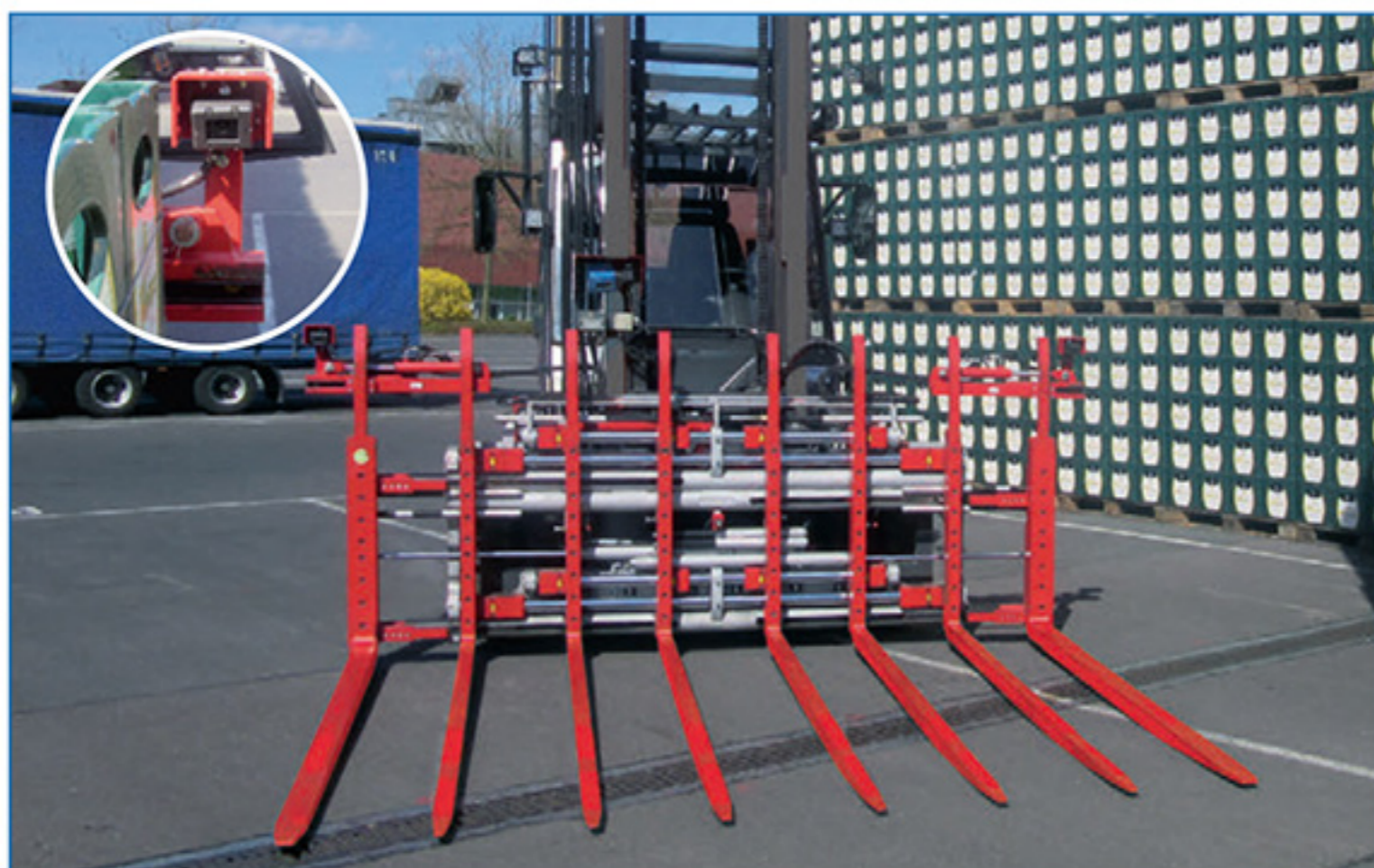
image shows APK 80-C with special equipment: telescopic camera
